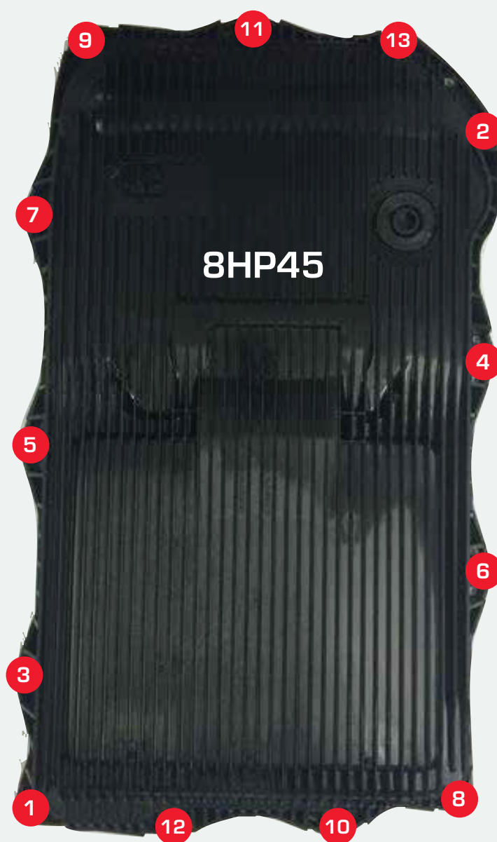
FIGURE 1 TIGHTENING TORQUE FOR SCREWS ON A PLASTIC OIL PAN = 10 Nm \pm 1.0 Nm.
